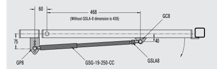
Suggested mounting positions for 90 degree opening of typical gate using a GSG-19 and GSG-22 fitted with a GSLA.
