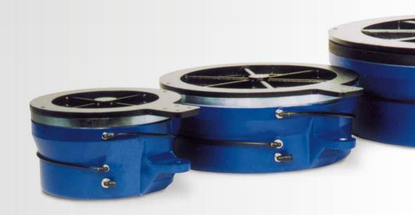
Standard PAL isolators have a natural frequency of up to  $1.7~{\rm Hz}-{\rm depending}$  on the height of the isolator. Even lower natural frequencies (up to  $0.5~{\rm Hz}$ ) are possible for isolators manufactured according to customer specifications.
