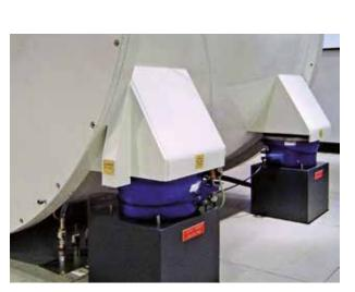
A measuring machine as an example of receiver isolation
