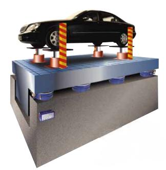
Test benches, example: street simulation test bench
