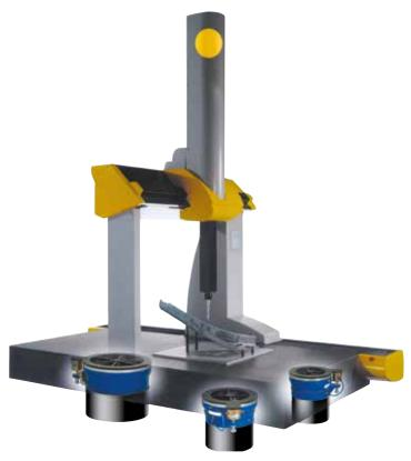
Measuring tables, example: coordinate measuring machine
