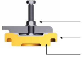
Lock screw is secured against the machine foot after the machine has been levelled out.
